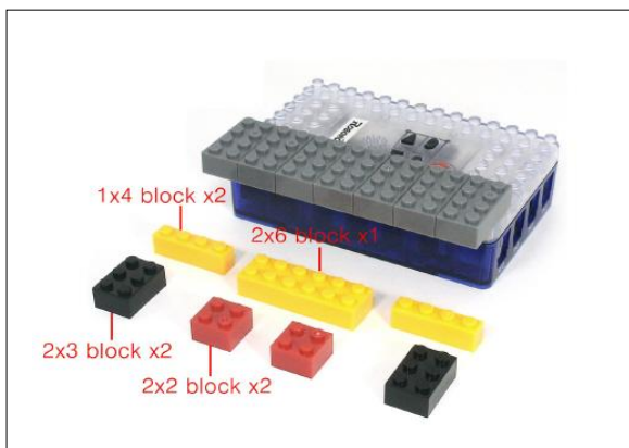
2. Assemble the 2x3, 2x2, 1x4 and 2x6 block with the CPU block.
