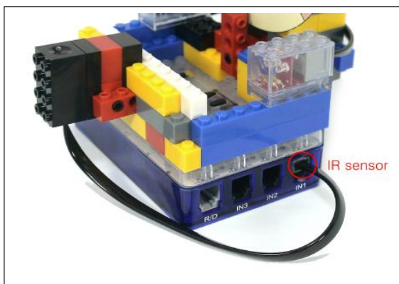
18. Using the 200mm cable, connect the infrared ray sensor to the IN1 of the CPU block. Now, Roulette-Bot is finished.
