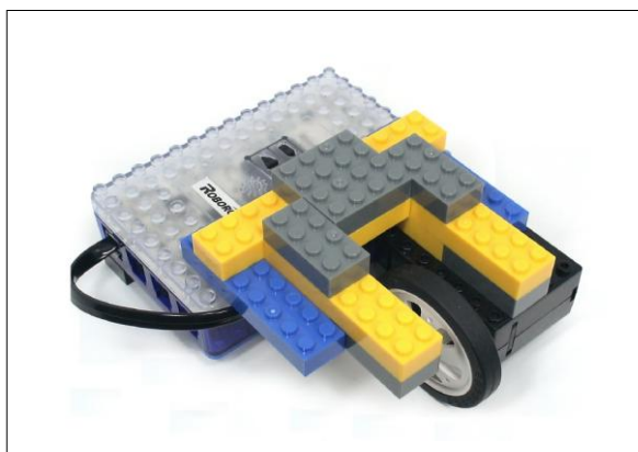
5. Assemble the 2x6 and 1x2 block with the structure of 4.
