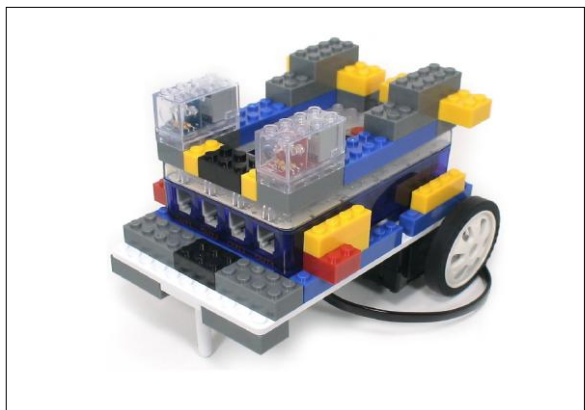
9. Insert the wheel to the DC motor, and then assemble the support block with the main block.
