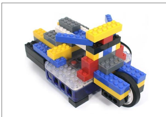
12. Plug the DC motor cable to the OUT1 of the CPU block.
