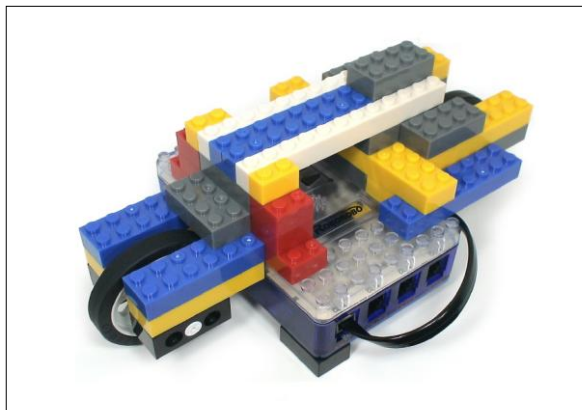
10. Assemble 1x8, 1x2 and 1x12, 2x4 block with the structure of 9.
