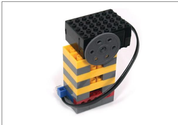
14. Assemble the wheel guide and DC motor with the structure of 13.
