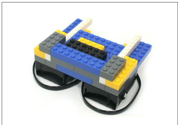
8. Assemble the 1x8, 1x4 and 2x3 block with the structure of 7.
