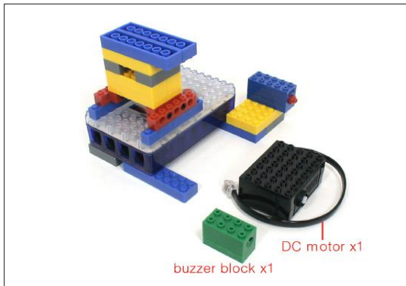
7. Assemble the buzzer block and DC motor with the upside of the structure of 6.
