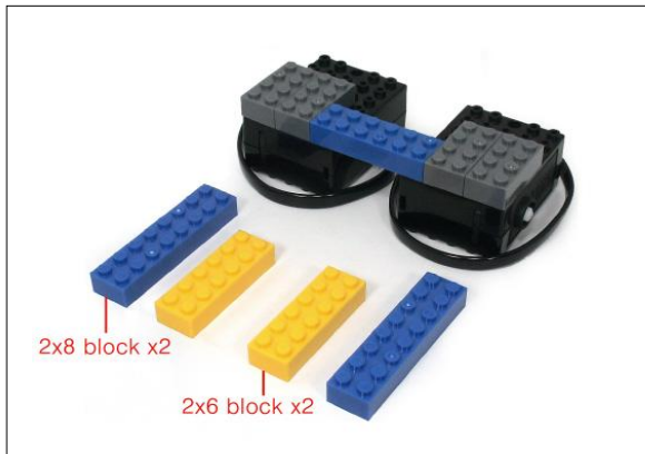
5. Assemble the 2x8 and 2x6 block with the DC motor.
