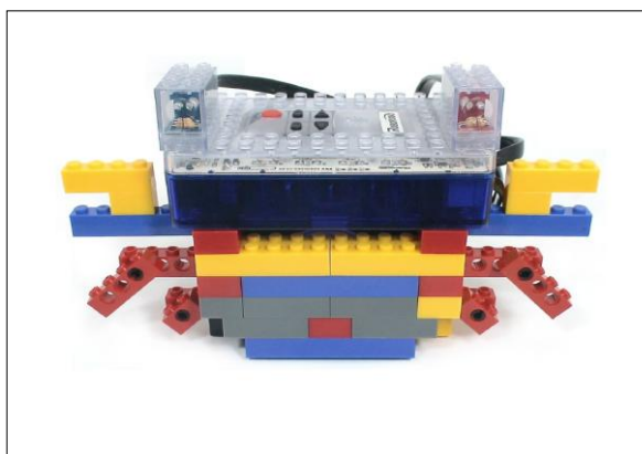
11. Connect the DC motor cable to OUT1 of the CPU block. Using the 200mm cable, Using the 200mm cable, connect the blue LED to OUT 2 of the CPU block, and red to OUT3.
